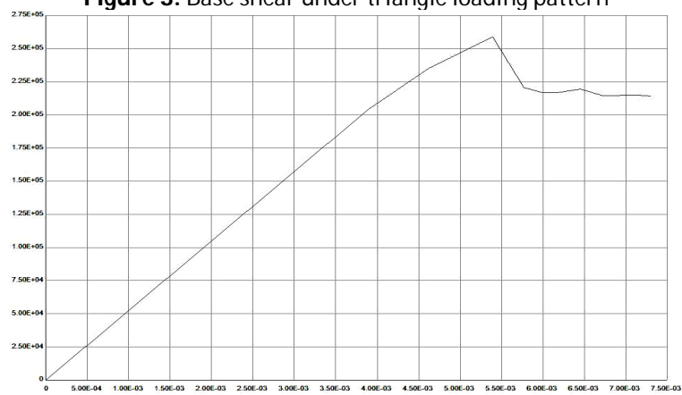
Figure 3: Base shear under suitable loading pattern with lateral forces
