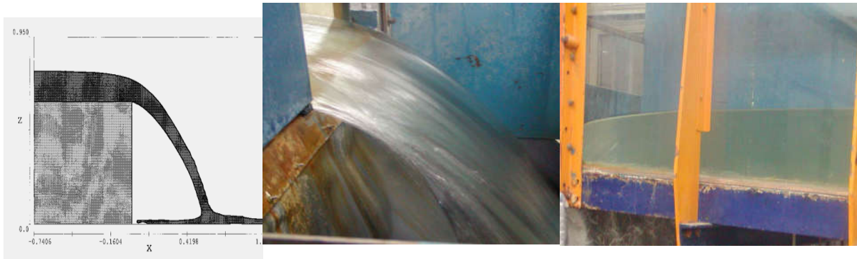
Fig. 1. (a) Snapshot of developing flow over a drop; (b) flow over a free overfall, and (c) free surface profile
