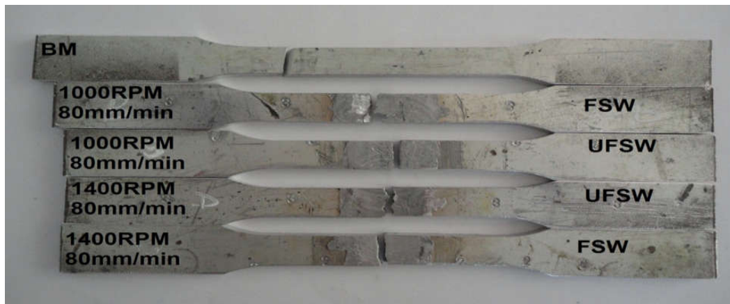
Figure 6. Fracture in weld joint at rotational speeds of 1000 and 1400 rpm in air or underwater conditions
