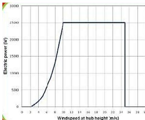
**Figure 2. Produced Power of the 660KW Turbine in Different Speeds**
