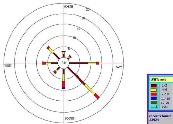
Figure 13. Wind Direction Distribution Curve in the Height of 10m
