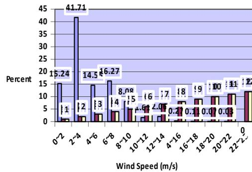
Figure 6. Percent of the Wind Speed in Each Interval for 2010 in the Height of 40m
