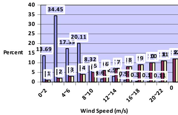
Figure 5. Percent of the Wind Speed in Each Interval for 2010 in the Height of 24m
