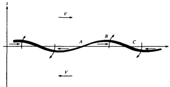
Figure 1. Kelvin Helmholtz instability. Two fluids movements in opposite directions causing turbulence in the flow
