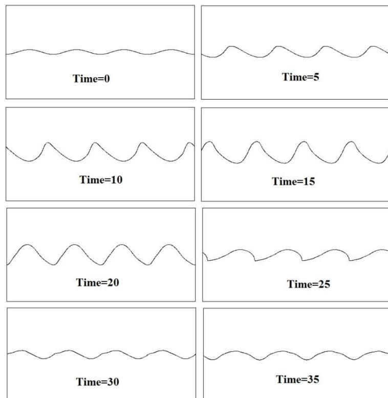
Figure 8. Kelvin Helmholtz instability and growth of disturbances acting on the interface of two different flows, density ratio = 10,  $Re_1 = 5000$ ,  $Re_2 = 1000$  and  $We=1.7$
