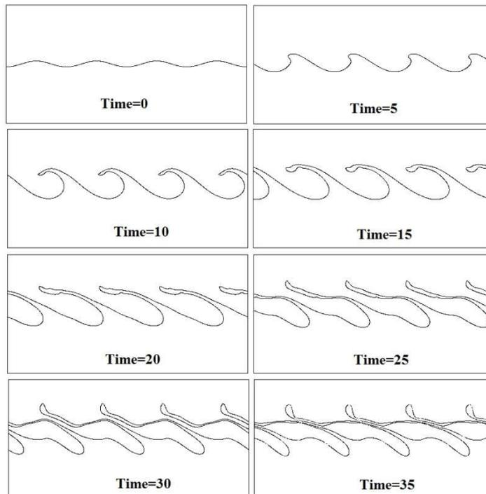
Figure 10. Kelvin Helmholtz instability and growth of disturbances acting on the interface of two different flows, density ratio = 10,  $Re_1 = 5000$  ,  $Re_2 = 1000$  and  $We=10.0$
