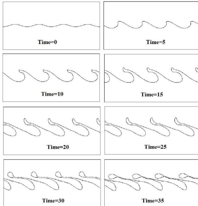
Figure 9. Kelvin Helmholtz instability and growth of disturbances acting on the interface of two different flows, density ratio = 10,  $Re_1 = 5000$  ,  $Re_2 = 1000$  and  $We=5.0$
