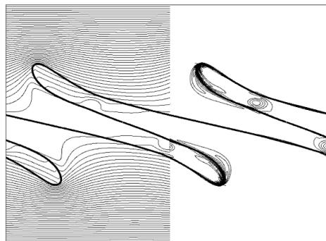
Figure 2. Deformation of the interface between two liquids due to surface tension and create finger
