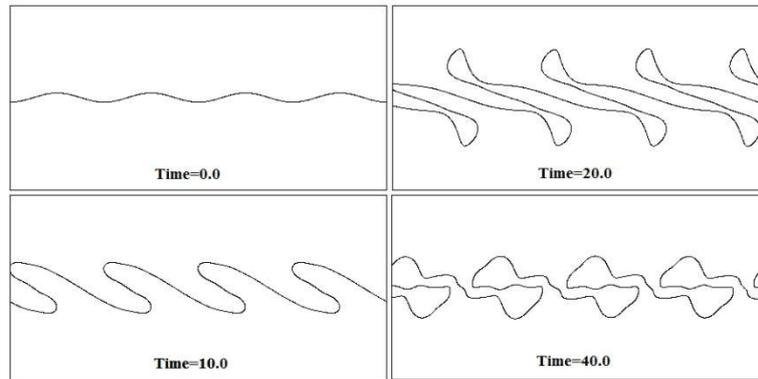
Figure 7. Kelvin Helmholtz instability and growth of disturbances acting on the interface of two similar flows for  $Re_1 = Re_2 = 10000$  and  $We=6.0$
