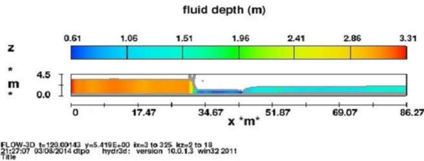
**Figure (2) fluid depth in 0.6m Aqili intake disruption**
