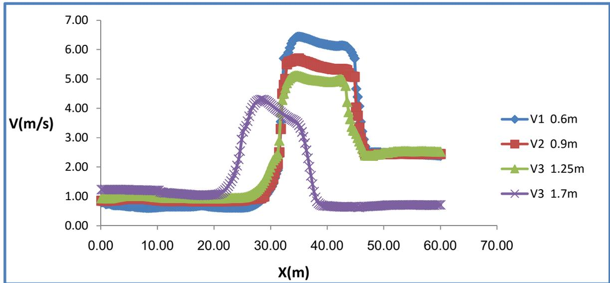
Figure (7) average velocity in Aqili intake four disruption modes (V average velocity, X length)
