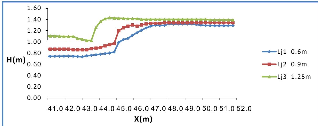
Figure (6) jump length comparison in Aqili intake (H fluid height, X length)
