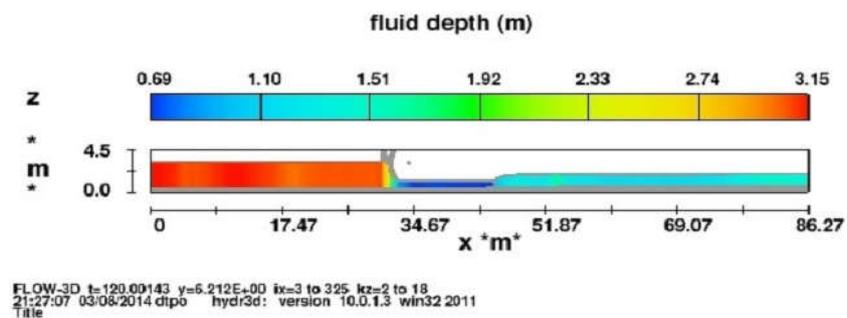
**Figure (3) fluid depth in 0.9m Aqili intake valve disruption**
