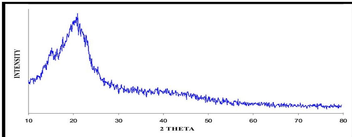
**Figure 2: XRD Pattern of Chitosan**
