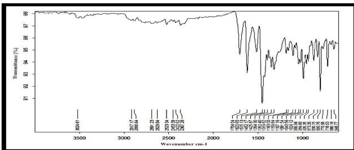
Figure 5: IR Spectra of Moxifloxacin
