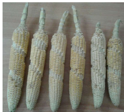
Fig. 3 Samples of kernels taken spirally over Dent corn and Sweetcorn cob to measure physical properties
