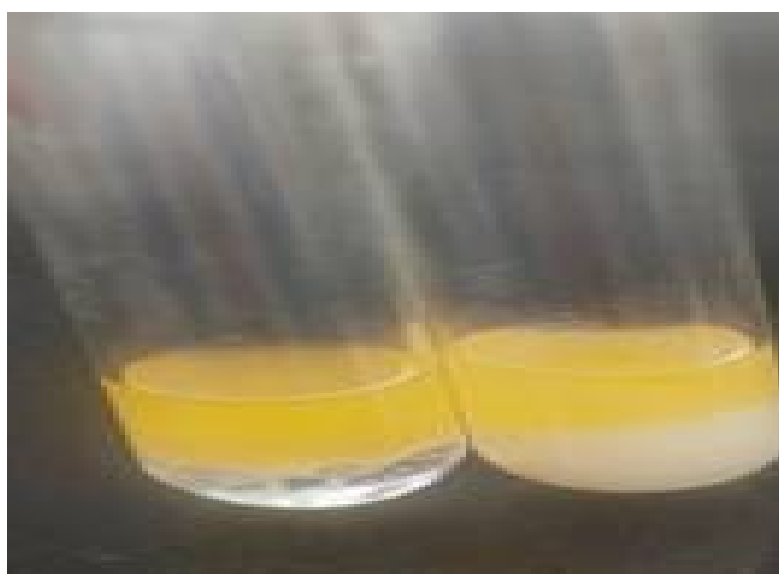
Photoplate 1: Emulsification of Engine Oil
