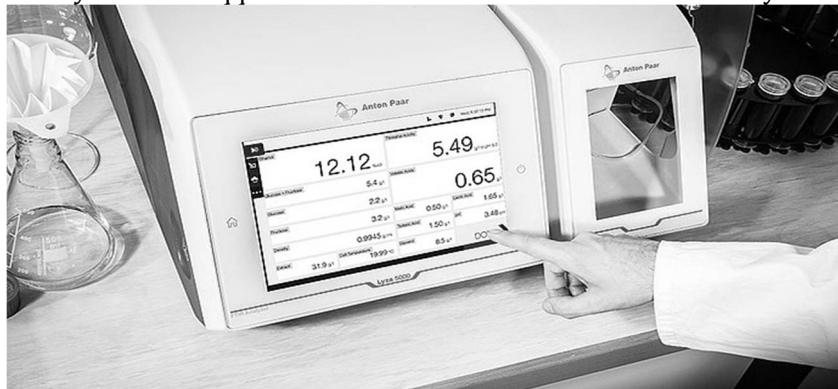
Fig.2FTIR Wine analyzer Lyza 5000 wine Sorce: Anton Paar
