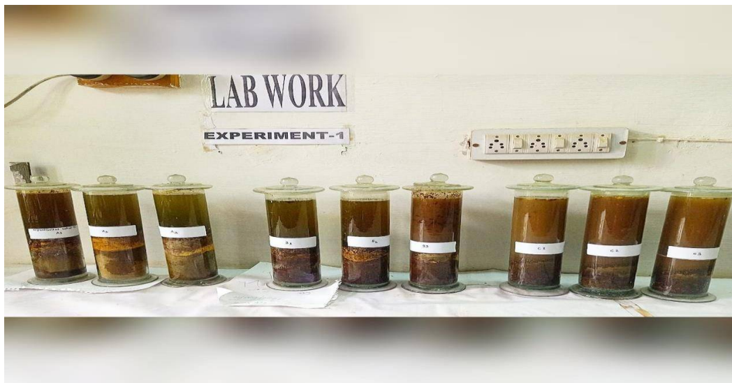
Figure 2. All the bioreactors after filling industrial waste water.
