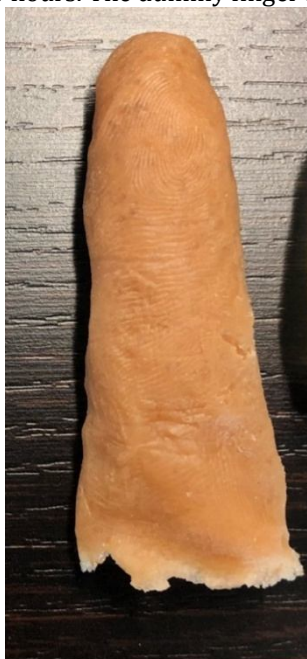
Fig 1: The final appearance of the dummy finger prepared with the aid of gelatin and glycerin.
