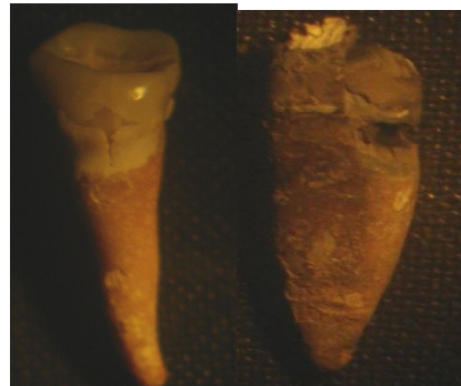
Fig.11 Detachment of dental amalgam restoration from crown, restoration still in shape, at an exposure of 850 ° C
