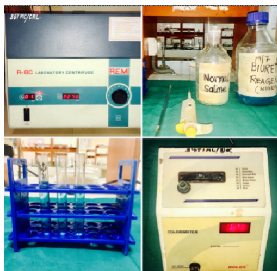
Fig 2: Armamentarium used for protein estimation A) Centrifuge machine B) Micropipette, normal saline and Biuret reagent C) Test tubes with rack D) Colorimeter
