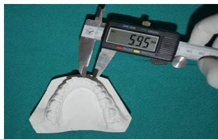
Fig.1: Digital calliper used to measure tooth dimension on study model with resolution of 0.01mm
