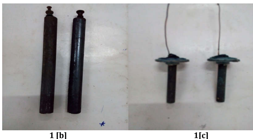
Photograph 1. [a] Design of MFC with electrode of different dimension, [b] carbon rod (length=15cm, dia =1.5 cm), [c] Carbon rod (length = 5cm, dia= 0.6 cm)
