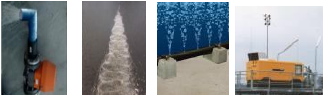
Figure 3- from the right 1 - the compressor station, 2 - pipe with special nozzles incorporated and anchor blocks, 3 - level generated by bubble curtains to the surface, 4 - the discharge valves on end of the nozzle tube.
