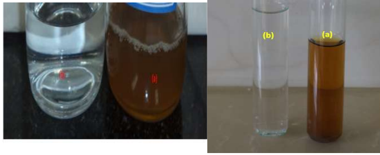
Figure1) Biosynthesis of silver nanoparticles observation by change color to brown.(a) silver nanoparticles formation as a test (b) silver nitrate as a control
