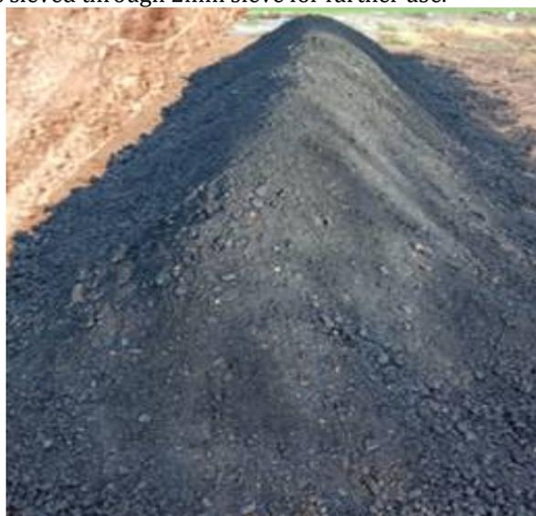
**Plate 4. Crushed tapioca stem waste biochar (TSWBC)**
