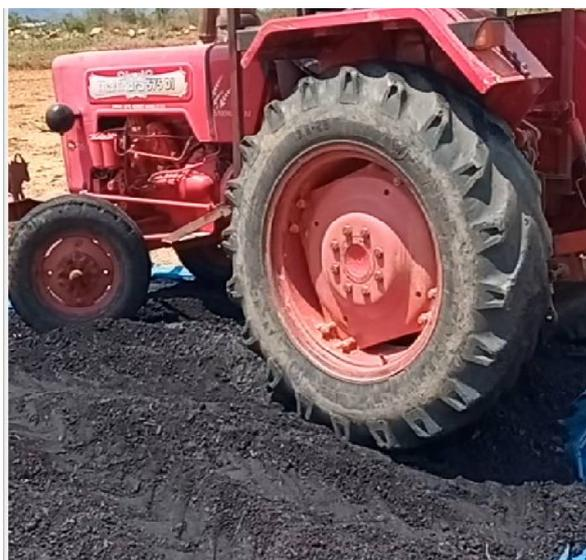
**Plate 3. Crushing of biochar by tractor**
