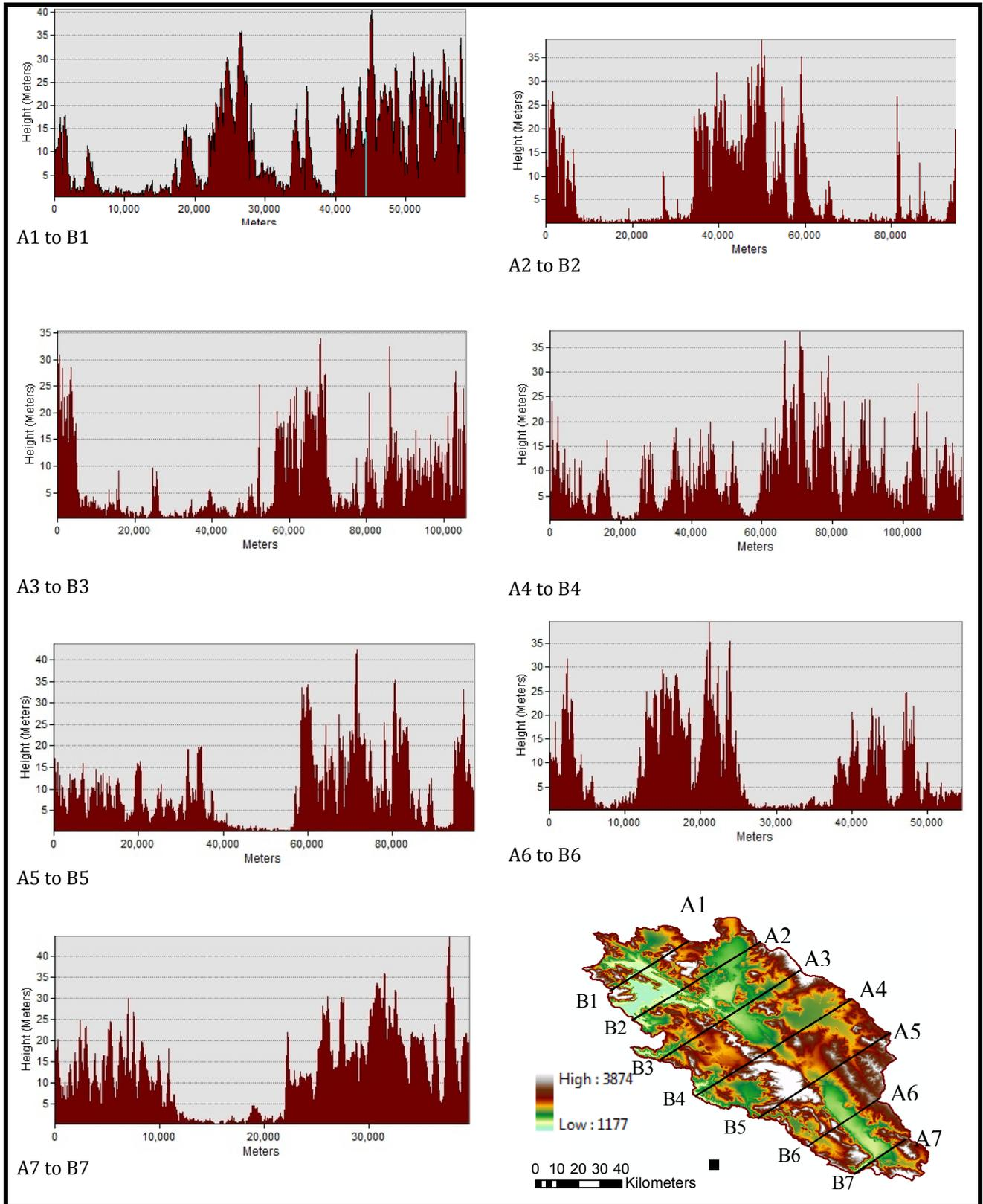
Figure 2: Cross-sections of watershed of Garin
