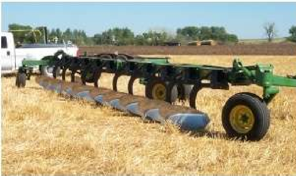
Figure 6. A large modern moldboard plow used in the north-central U.S. agricultural production areas.
