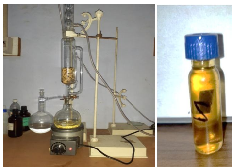
Figure 2: Soxhlet extraction of S. emarginatus seed kernel & extracted oil sample for GC-MS Analysis
