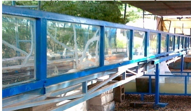
Figure (2) A view of the 13 m flume
