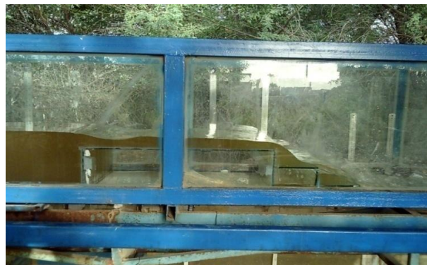
Figure (3) A view of the spillway with 3 steps, 20 cm height and a slope of 1: 2
