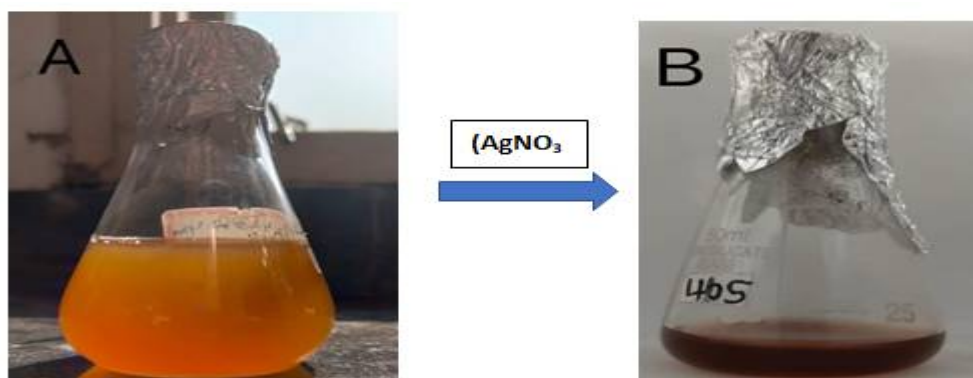
Figure: 1 Colour change of reaction solutions (A) moringa oleifera leaves extract (B) Ag nanoparticles solutions
