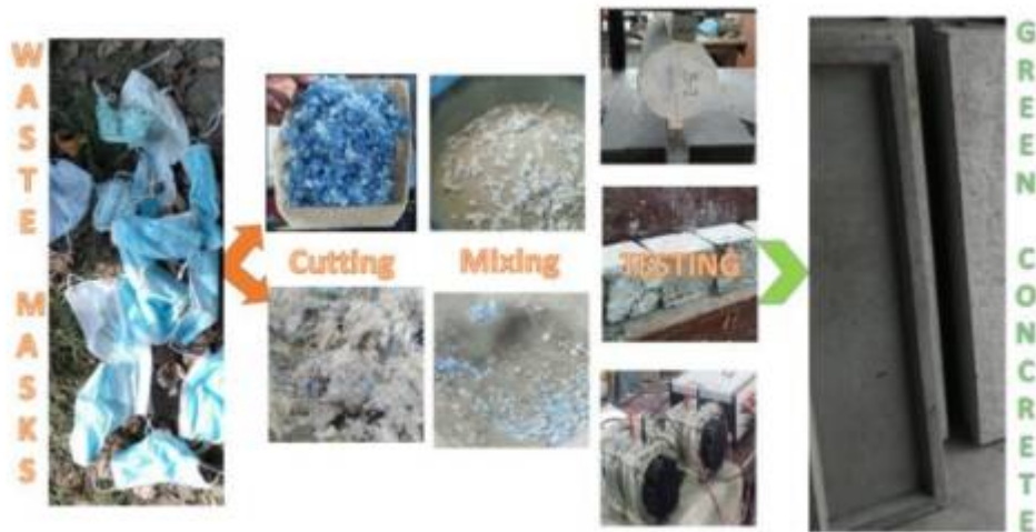
figure 1 :Methodology to use waste masks in concrete.
