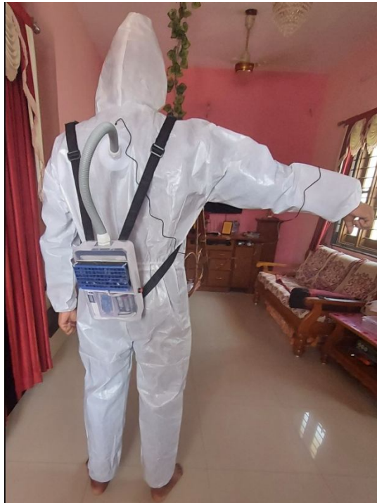
Figure 7: Air Conditioning Unit attached to PPE kit.
