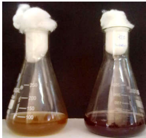
Figure 3: Ag-NPs cell filtrates of A. niger with \text{AgNO}_3 (Right) and Positive control (Left)
