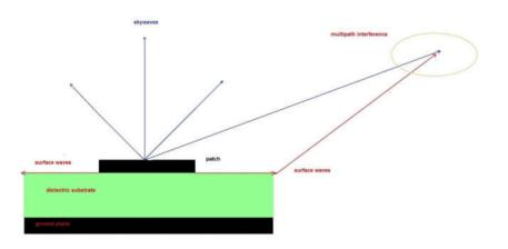
Figur4:Sky waves, surface waves and multipath interference in patch antenna.
