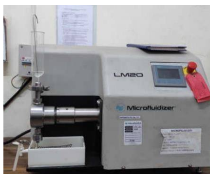
Figure 1: Micro fluidizer used in the formulation of Sulindac-loaded Nano emulsion
