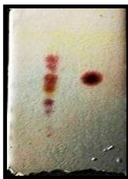
Figure 1. TLC plate showing spots having different Rf values (0.85, 0.79, 0.61, 0.55, 0.41 & 0.35) of methanolic extract of E. officinalis fruits
