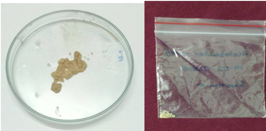
Fig. 15 BC produced by Acetobacter sp. in sugarcane bagasse hydrolysate (a) Wet BC (b) Dry BC
