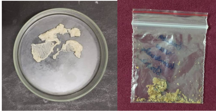
A B Fig. 10 BC produced by K. xylinus (a) Wet BC (b) Dry BC
