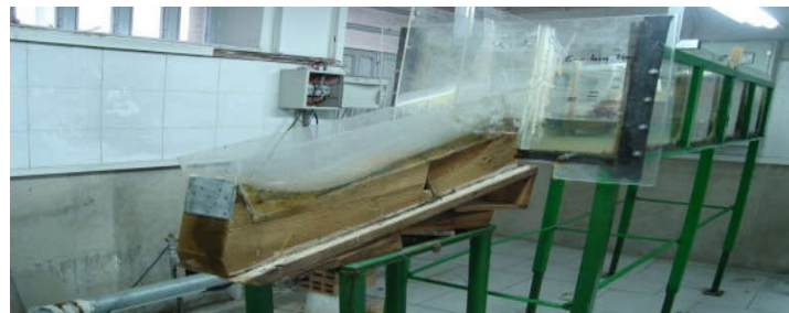
Figure (3): Laboratory model of Balarud Dam spillway
