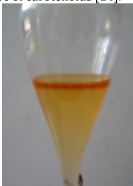
Figure 2: Phase separation of pigment with diethyl ether
