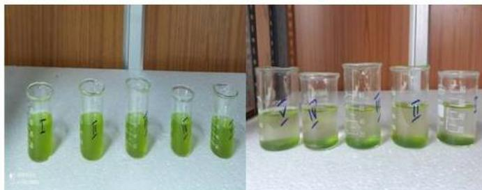
Fig. 4 Jar test – Before flocculation Fig. 5 After flocculation
