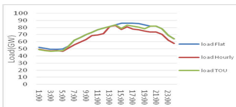
Figure 5: comparing the consumption based on the Flat, Hourly and TOU pricing strategies
