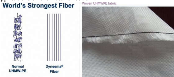
Figure 1: (a) Dyneema woven Fibers (b) comparing Dyneema fibers with conventional fibers Dyneema fibers are supplied in various types and for wide different applications. HB type is used in constructing armored sections of combat aircrafts, ships, and troop carriers. These fibers are extremely resistant to heat and have very low flammability limit. Moreover, their textures are such that prevent shrapnel, debris, and particles from be scattered around after the projectiles shot from military arms hit the surface[6]. Dyneema of HB25 type has been used in the present study. Besides, composite panels consisting fibers and resin are highly important, therefore a wide range of studies have been done on this field. When the number of textiles (lamina) is low, better strength will be achieved in dry mode, but when thickness increases density will increase accordingly. When resin is incorporated in the panels, flexural strength will increase and it leads to higher efficiency. Addition of resin can improve the strength through four mechanisms[7,8]:
