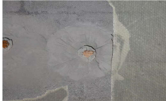
Figure 8: Reaction bonded silicon carbide ceramic fracture after ballistic test
