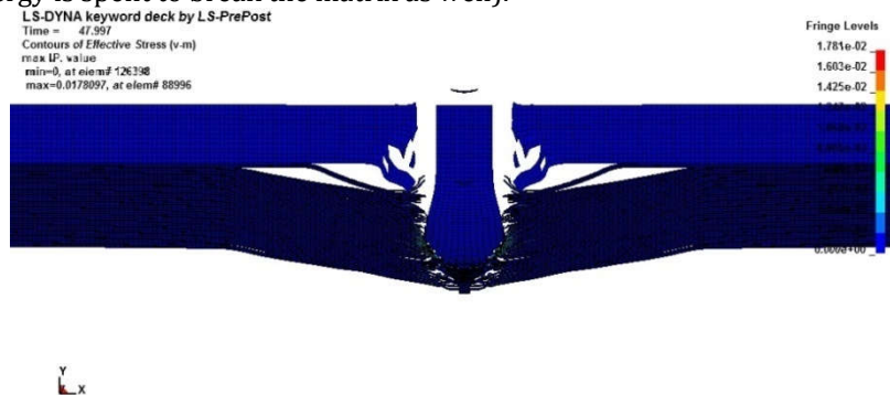
Figure 5: Fracture of composite first layers inside the RBSIC1 armor prior to deformation and meeting fracture strain at the moment of 48 \mu s
