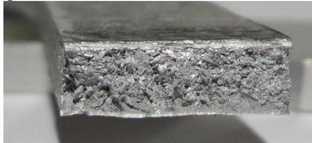
Figure 3. Fracture cross-section of the welded sample underwater
