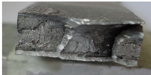
Figure 4. Fracture cross-section of the air welded sample
