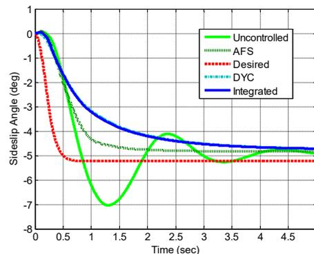
**Figure (13) Side slip angle of the fixed steering maneuver on dry roads**
