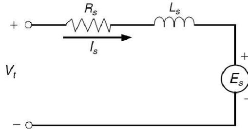
Figure 7 A single-phase electric BLDC model equivalent circuit [9]
