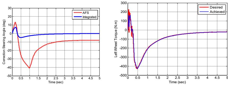
**Figure (16) Steering correction angles of the front wheels of the fixed steering maneuver on dry roads**
