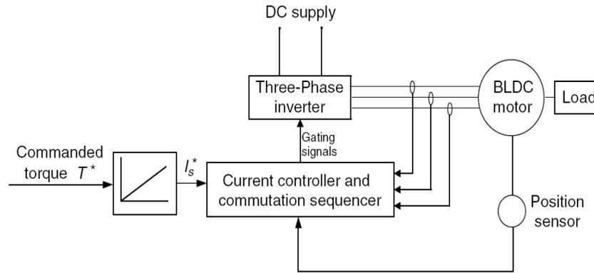
**Figure 11 Block diagram of the three-phase BLDC electric motor torque control**
