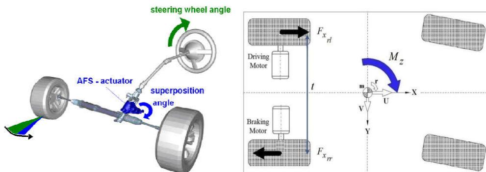
**Figure 1 Front wheels active steering system by total spin solar gear**
