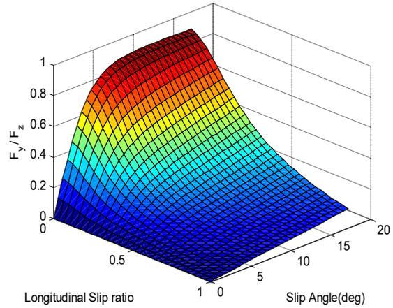
**Figure 6 Normalized transverse force diagram in terms of the lateral slip angle and longitudinal slip**
