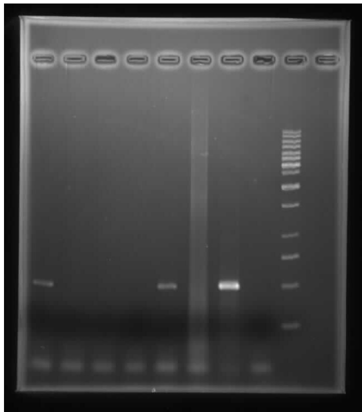
Picture2-Electrophoresis of PCR tests on blood samples of bovine tuberculosis in cattle infected
