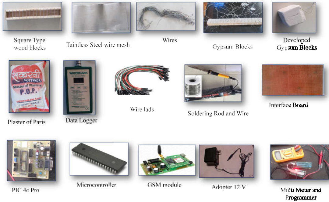
Fig. 1. Different components used for fabrication and developing the gypsum block soil moisture sensing system
