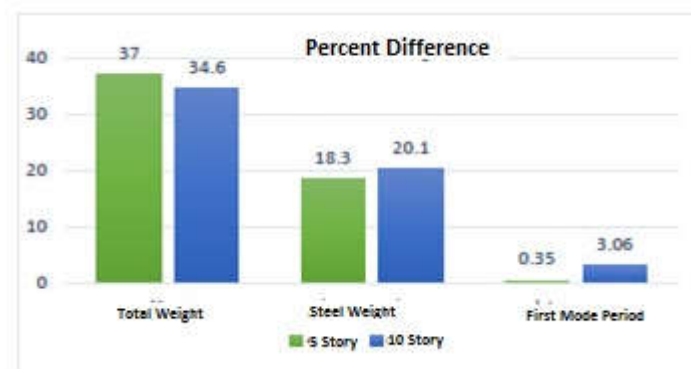
Chart1. Comparison of reductions in different parameters as a result of using modern materials in research model
