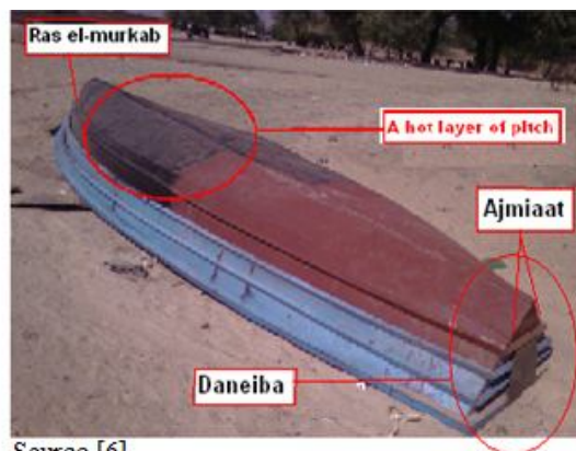
Plate 9. Depicts a hot layer of pitch painted on back of fishing boat's bottom for tightness
