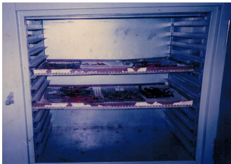
Fig. 2. View of trays were placed in the cabinet dryer in the perforated trays
