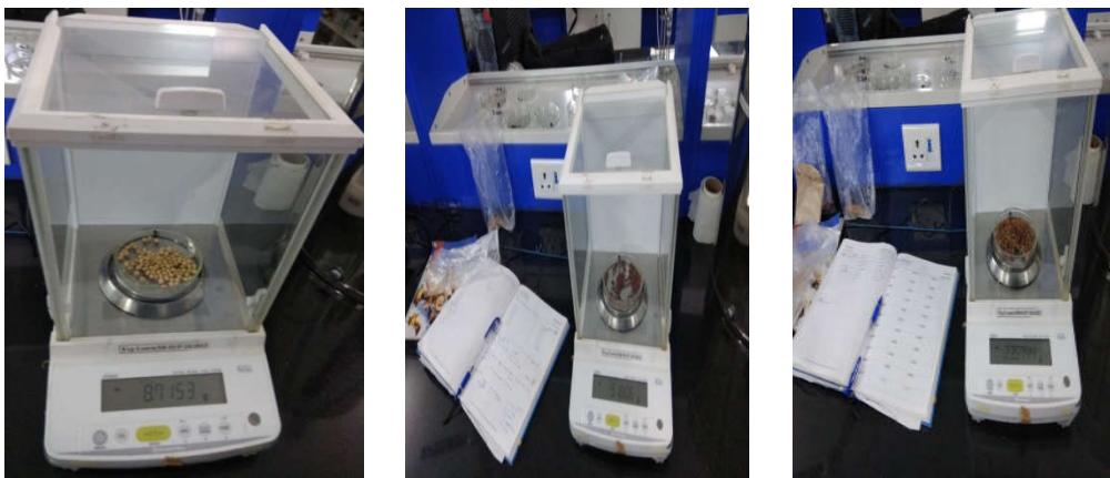
Fig.2 Test weight of Soybean, pigeonpea and chickpea by digital weighing balance
