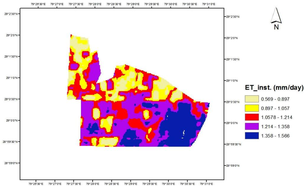
**Fig. 9.** Instantaneous Evapotranspiration Loss (mm/ day) at Study Area
