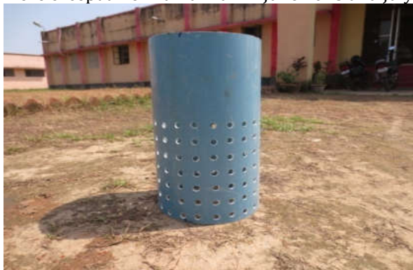
Fig. 1: Perforated PVC water tube used for observation of water level by farmers
