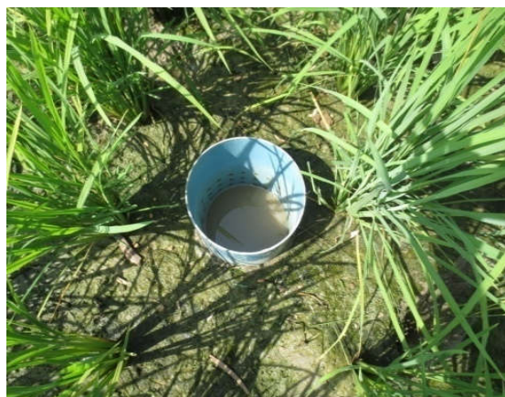
Fig. 3: Depleting water level at 5 cm below soil surface: Time to irrigate the paddy field in T02
