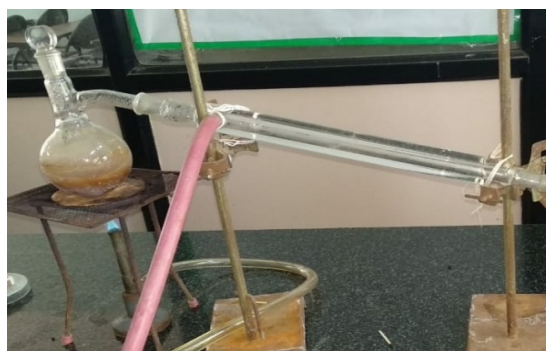
Figure 2: Distillation process in distillation assembly
